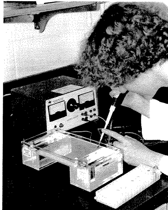
Figure 11.3 A scientist is using a micropipette to load a DNA sample into an agarose gel. The gel is in an electrophoresis chamber full of buffer. The power supply for the chamber is on the laboratory bench behind the chamber.
